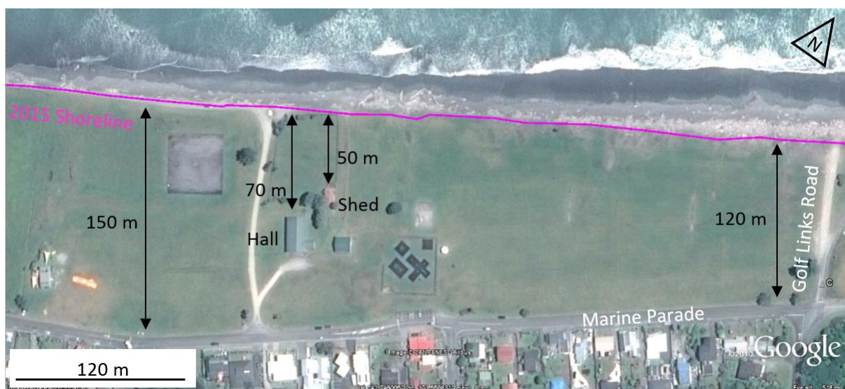
Figure 4-1: Features and facilities on Carters Beach domain reserve. Measurements show distance inland from 2015 shoreline position. Between 4 and 10 m of additional retreat has occurred in the 18 months since this photograph was taken. [Credit: Google Earth, Imagery Date: 25/12/2015].
